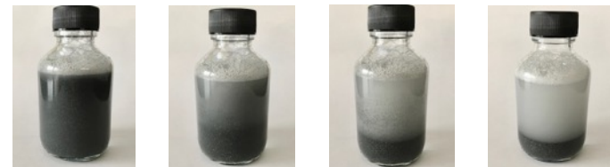
Metallic car paint diluted 1:3 in an INARCO cleaning solution.
